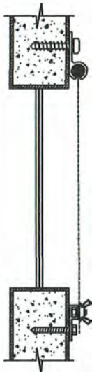
C-Channel (top) F-Track (bottom) Typical Vertical Window Sectional View
