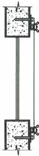
F-Track Typical Vertical Window Sectional View
