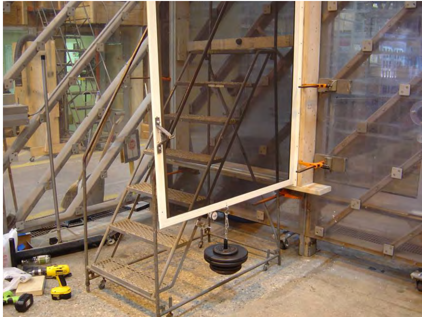
Photo No. 3 Test Setup of Sag Test
